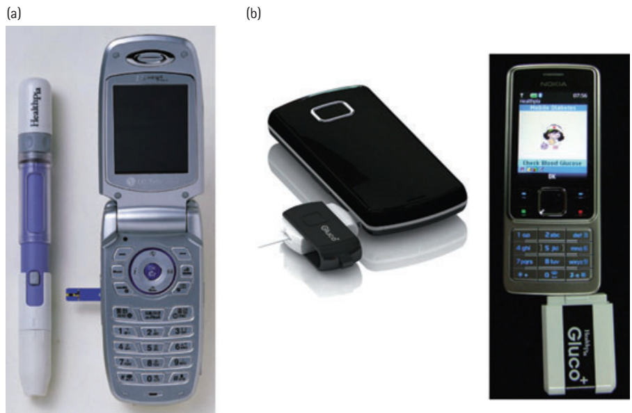
Figure 58.2 Glucometer with telecommunication. Adapted from Cho et al. [41]. (a) The Diabetes Phone (Healthpia, Korea) has a glucometer in a battery pack (phone embedded type). (b) The glucometer can be directly connected to a cellular phone (Dongle type). (Gluco plus, Healthpia, Korea.)
