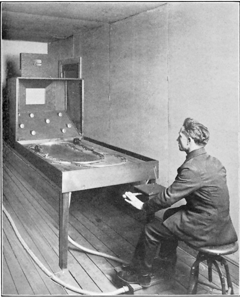
A 1920s example of work sample testing: an apparatus to test the skills of prospective trolley drivers.
