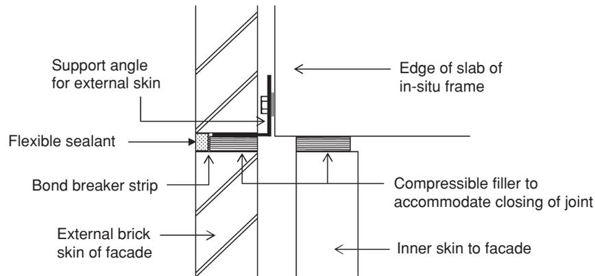
**Figure 12.2** Brick façade on reinforced concrete frame – detail of movement joints.
