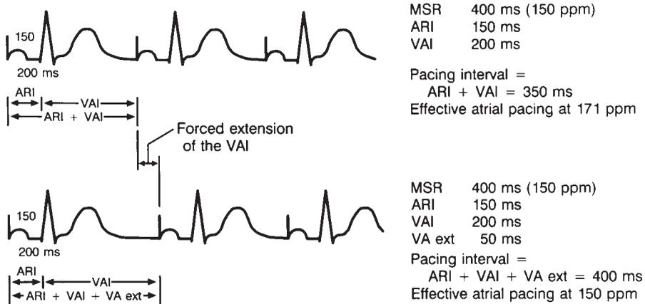
**Figure 6.44.** Pacing at MSR. Timing algorithm provides effective pacing at MSR with intrinsic conduction to the ventricle. ARI = interval from atrial stimulus to sensed R wave; VA = ventriculoatrial; VAI = ventriculoatrial interval. (From Hayes DL, Ketelson A, Levine PA, et al. Understanding timing systems of current DDDR pacemakers. *Eur JCPE* 1993;3:70–86. By permission of Mayo Foundation.)
