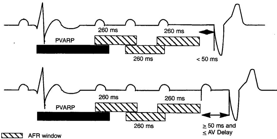
**Figure 6.36.** Atrial Flutter Response. Atrial detection inside PVARP starts a 260-ms interval which will restart if another atrial event is detected. A ventricular pace will take place on the scheduled interval. An atrial pace will not occur unless there is at least 50 ms before the scheduled V pace. This prevents competitive pacing. (Courtesy of Guidant Corporation.)
