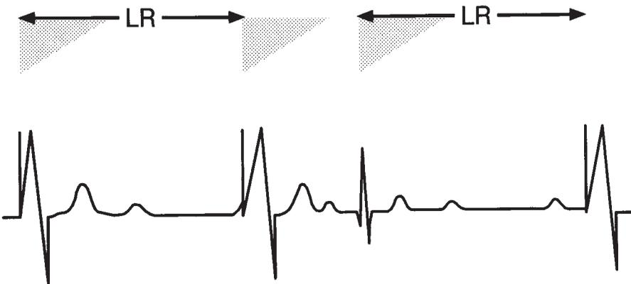
**Figure 6.3.** The VVI timing cycle consists of a defined LRL and a VRP (*shaded triangles*). When the LRL timer is complete, a pacing artifact is delivered in the absence of a sensed intrinsic ventricular event. If an intrinsic QRS occurs, the LRL timer is started from that point. A VRP begins with any sensed or paced ventricular activity.
