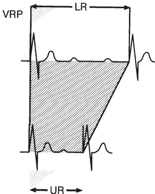
**Figure 6.8.** The VVIR timing cycle consists of an LRL, an upper rate limit (UR), and a VRP, represented by shaded triangles. As indicated by sensor activity, the VV cycle length shortens accordingly. (The striped area represents the range of sensor-driven VV cycle lengths.) In most VVIR pacemakers, the VRP remains fixed despite the changing VV cycle length. In selected VVIR pacemakers, the VRP shortens as the cycle length shortens.
