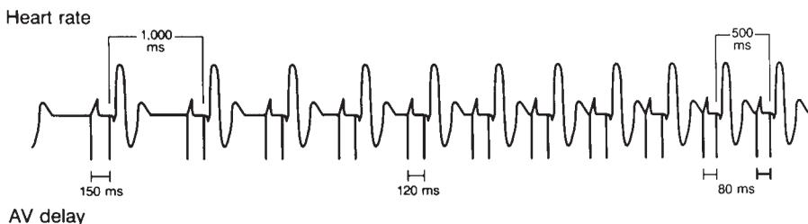
**Figure 6.20.** As heart rate increases, AV delay dynamically adapts to the change in cycle length. (From Hayes DL, Ketelson A, Levine PA, et al. Understanding timing systems of current DDDR pacemakers. *Eur JCPE* 1993;3:70-86. By permission of Mayo Foundation.)
