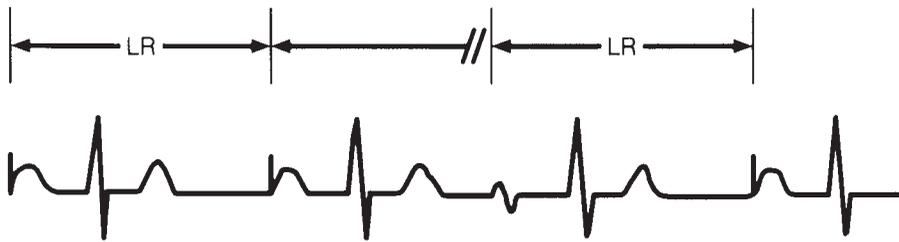
**Figure 6.5.** The AAI timing cycle consists of a defined LRL and an ARP. When the LRL timer is complete, a pacing artifact is delivered in the atrium in the absence of a sensed atrial event. If an intrinsic P wave occurs, the LRL timer is started from that point. An ARP begins with any sensed or paced atrial activity.
