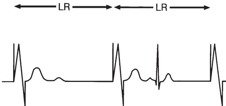
**Figure 6.1.** The VOO timing cycle consists of only a defined rate. The pacemaker delivers a ventricular pacing artifact at the defined rate regardless of intrinsic events. In this example, an intrinsic QRS complex occurs after the second paced complex, but because there is no sensing in the VOO mode, the interval between the second and the third paced complex remains stable.
