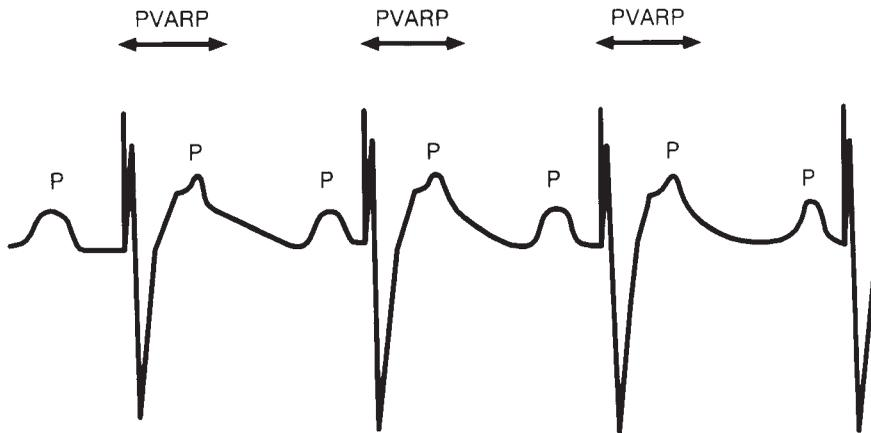
**Figure 6.30.** In the DDD pacing mode, the programmed upper rate limit (UR) cannot be violated regardless of the sinus rate. When a P wave is sensed after the PVARP, the AVI is initiated. If, however, delivering a ventricular pacing artifact at the end of the AVI would violate the UR, the ventricular pacing artifact cannot be delivered. The pacemaker would wait until completion of the UR and then deliver the ventricular pacing artifact. This action would result in a prolonged AVI.
