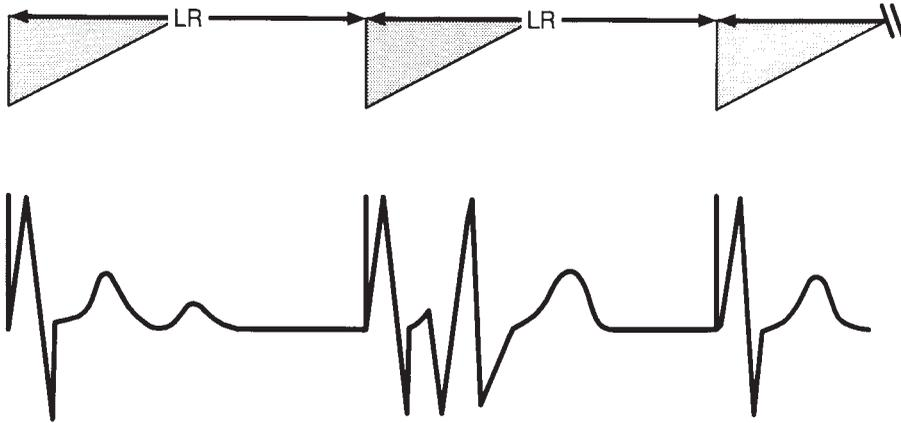
**Figure 6.4.** If, in the VVI mode, a ventricular event occurs during the VRP (*shaded triangles*), it is not sensed and therefore does not reset the LRL timer.
