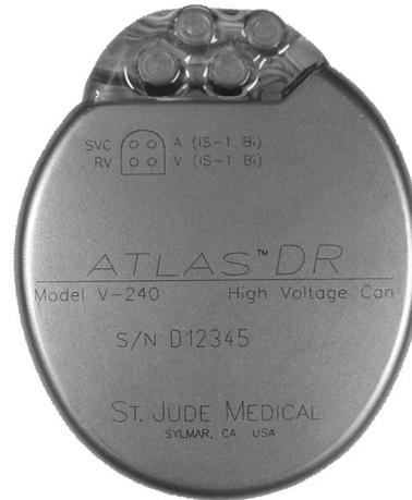
**Figure 1.7** Defibrillator pulse generator.
