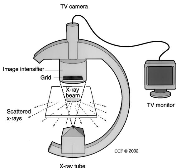
**FIGURE 3-7.** Essential components of C-arm type fluoroscopy units.
