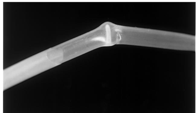
**FIGURE 3-1.** Working channel of the flexible bronchoscope. This channel has been damaged by a needle, and the accumulation of debris in the defect will prevent effective cleaning. A positive leak test led to its discovery.
