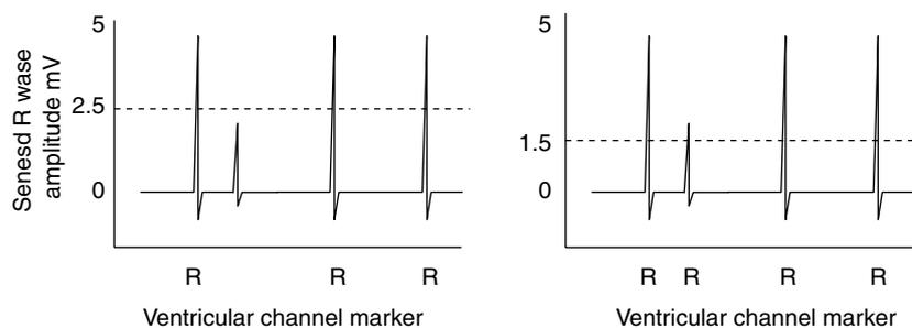
**Figure 1.12** The second intrinsic complex (a PVC) does not create a large enough signal to be sensed in the ventricular channel with the sensing set at 2.5 mV (dotted line). Therefore, the pacemaker does not recognize the presence of the second intrinsic R wave. (The marker channel at the bottom indicates which intrinsic R waves are sensed by the pacemaker.) If the sensitivity (i.e. the threshold for sensing) had been lowered to 1.5 mV, the second beat would have been sensed.
