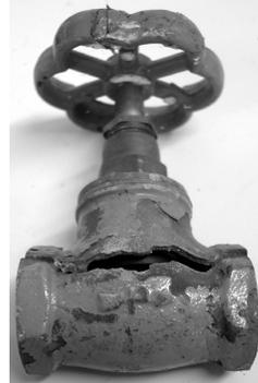
Frost damage to valve (causing wastage of water)
