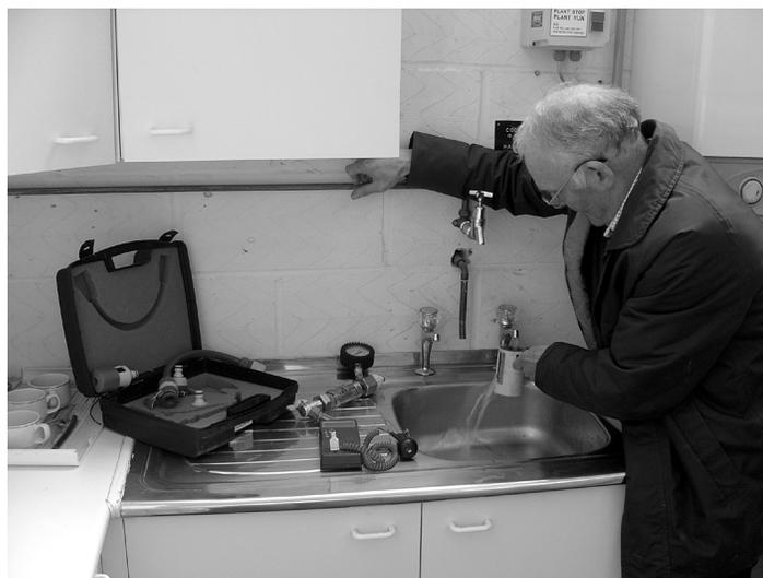
Operative taking water flow, pressure and temperature measurements
