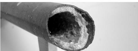
Section of pipe with evidence of limescale
