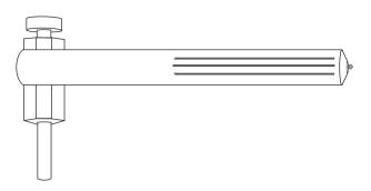
Figure 3.42 Manual torque driver
