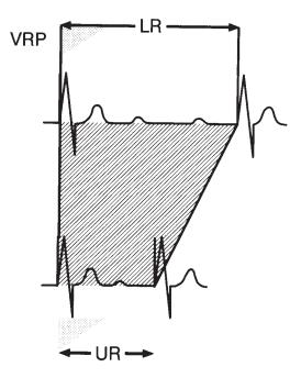
**Figure 6.8.** The VVIR timing cycle consists of an LRL, an upper rate limit (UR), and a VRP, represented by shaded triangles. As indicated by sensor activity, the VV cycle length shortens accordingly. (The *striped area* represents the range of sensor-driven VV cycle lengths.) In most VVIR pacemakers, the VRP remains fixed despite the changing VV cycle length. In selected VVIR pacemakers, the VRP shortens as the cycle length shortens.
