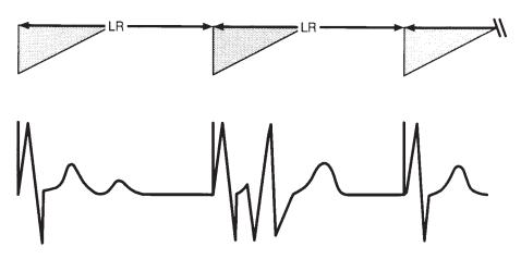
Figure 6.4. If, in the VVI mode, a ventricular event occurs during the VRP (shaded triangles), it is not sensed and therefore does not reset the LRL timer.
