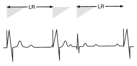
**Figure 6.3.** The VVI timing cycle consists of a defined LRL and a VRP (*shaded triangles*). When the LRL timer is complete, a pacing artifact is delivered in the absence of a sensed intrinsic ventricular event. If an intrinsic QRS occurs, the LRL timer is started from that point. A VRP begins with any sensed or paced ventricular activity.
