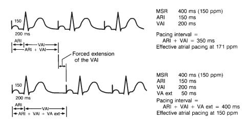
**Figure 6.44.** Pacing at MSR. Timing algorithm provides effective pacing at MSR with intrinsic conduction to the ventricle. ARI = interval from atrial stimulus to sensed R wave; VA = ventriculoatrial; VAI = ventriculoatrial interval. (From Hayes DL, Ketelson A, Levine PA, et al. Understanding timing systems of current DDDR pacemakers. Eur JCPE 1993;3:70–86. By permission of Mayo Foundation.)
