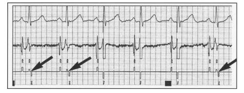
**Figure 6.17.** Surface ECG, atrial electrogram, and event markers (*arrows*) demonstrating occasional AR complexes, events that are occurring within the ARP. They coincide with the QRS complex but are detected on the atrial channel before being detected by the pacemaker on the ventricular channel.
