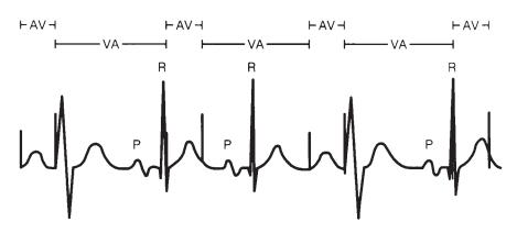
**Figure 6.2.** The DOO timing cycle consists of only defined AV and VV intervals. The VAI is a function of the AV and VV intervals. An atrial pacing artifact is delivered, and the ventricular artifact follows at the programmed AVI. The next atrial pacing artifact is delivered at the completion of the VAI. The intervals do not vary because no activity is sensed; that is, nothing interrupts or resets the programmed cycles.
