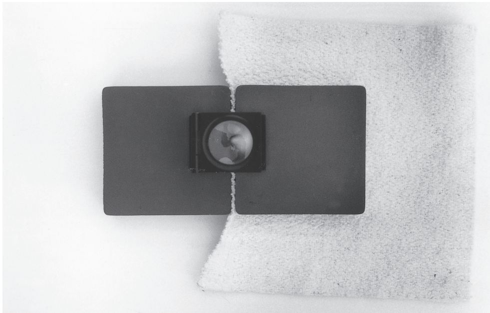
Figure 8 Measuring thickness. A method suitable for student practice. A 20 cm square of fabric placed between blocks and measured with a magnifying glass marked in mm.
