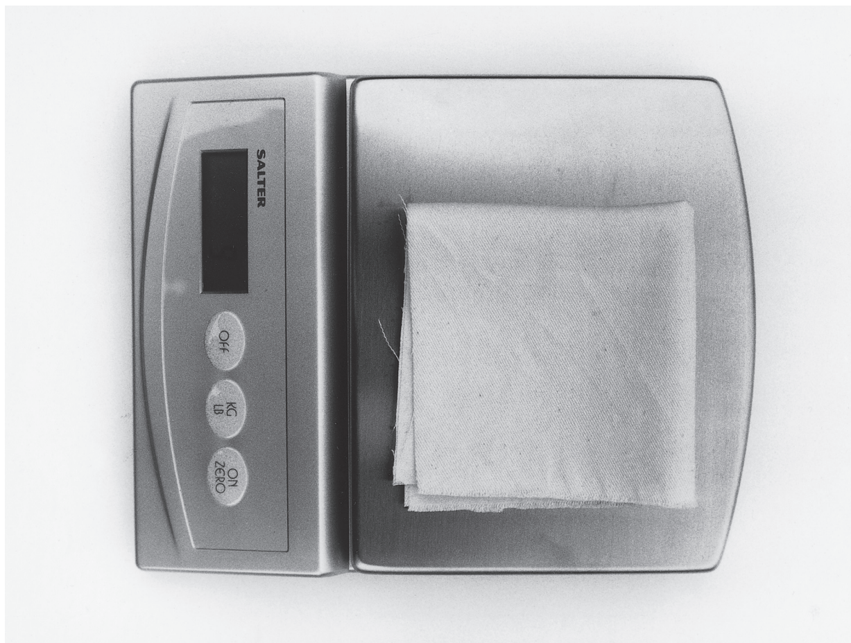
Figure 7 Measuring weight. A method suitable for student practice. A 20 cm square of fabric measured on a domestic scale that records in 1 gm intervals.
