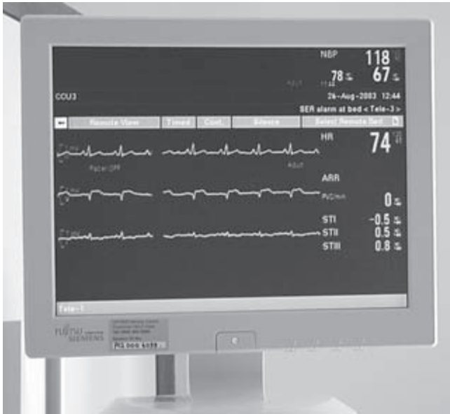
Fig. 8.1 Monitor displays three leads and ST segment monitoring.
