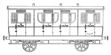
**Figure I.4** Montelius's figure 76: another of the first train-cars ordered for the Swedish state railways (made in Germany shortly after the mid-1850s): for first-and second-class passengers
