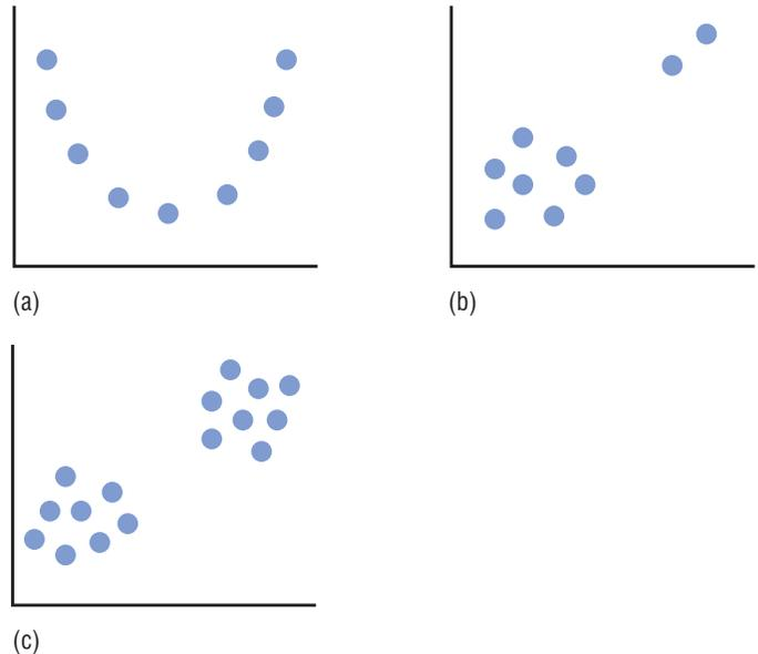
**Figure 26.2** Diagrams showing when it is inappropriate to calculate the correlation coefficient. (a) Relationship not linear,  $r = 0$ . (b) In the presence of outlier(s). (c) Data comprise subgroups.
