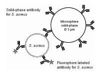
Microspheres used as solid-phase reaction carriers for bioaffinity assay. Three-component immunocomplexes are formed on the solid-phase surface in proportion to the analyte concentration.
